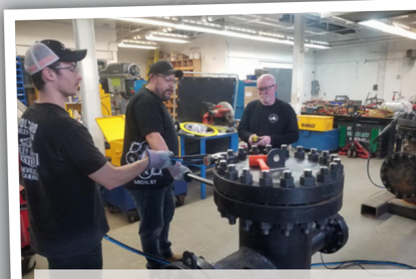
(Left to right) Local 67 training instructor Chris Legris, Training Coordinator Dale McGavin and member Doug Hynes work on controlled bolting in the local's training centre in 2023.
